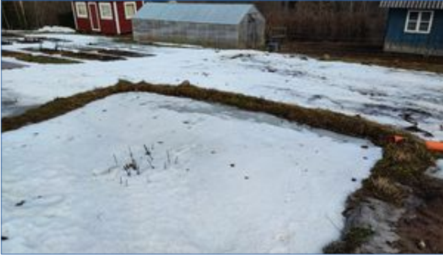
Figure 4: Nordic Botanical Ltd. test rain garden in winter 2024. All the area is frozen and covered with 10 - 15 cm of ice.
