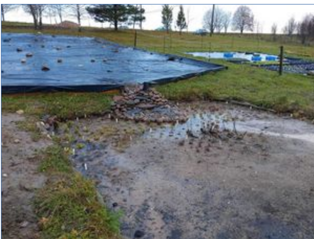
Figure 3: Nordic Botanical test rain garden during mid-winter snowmelt. The ground is frozen and does not let water to infiltrate.
